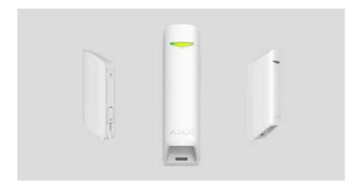
**MotionProtect Curtain** is a curtain type wireless motion detector. The detector has a narrow horizontal detection angle and is designed for indoor perimeter control: windows, doorways, and other entrances or exits of the guarded facility. Maximum motion detection distance is 15 m.
